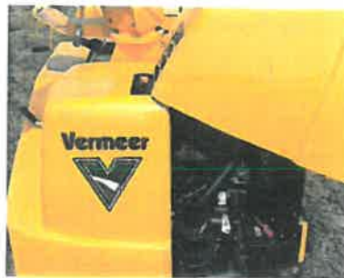
An optional sound-abatement package offers a combination of an engine shield liner, a triple-layer infeed curtain, and a sound-reducing coating on the discharge chute.
