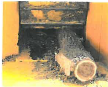
A large rectangular 12" x 17" (30 cm x 43 cm) feed opening helps boost productivity by reducing the need to trim material before it is fed into the chipper.
