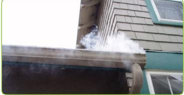
The City of Lansing is continuing efforts to repair the city's aging sanitary sewer system. In the next several weeks, customers may notice smoke coming from their sanitary sewers. This is part of a test to find leaks in the system. The non-toxic, odorless smoke is blownintosewermanholes, goesthrough the pipes, and comesout where there are broken pipes or where roof downspouts, outside area drains, or foundation drains are connected to the sanitary sewers.
